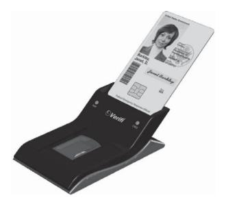
Insert SmartCard face up. Insert completely until the card indicator light illuminates. Removal of smart card can be accomplished by using the thumb and index finger and pushing against the smartcard extraction platform located in the backside of the device.
