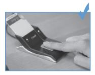
PROPER FINGER PLACEMENT Finger is flat to surface and centered in sensor area.
