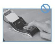
IMPROPER FINGER PLACEMENT Finger is not flat to surface and/or not placed in center of sensor area.
