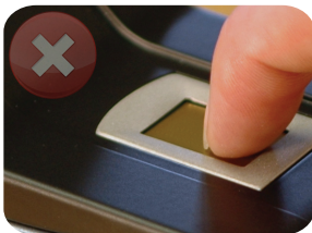
IMPROPER FINGER PLACEMENT Finger is not flat to surface.
