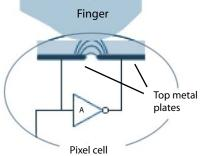
Active capacitive pixel-sensing technology
